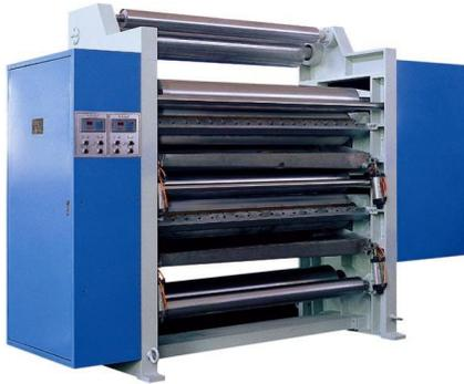
\*The high precision engraved applicator roll ensures even adhesive application and less amount of adhesive consumption.
